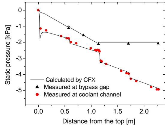
Fig. 4. The predicted and measured static pressure distribution.
