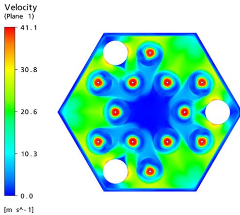
Fig. 3. The calculated velocity contour at the cross flow gap.
