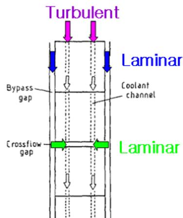
Fig. 2. Flow characteristics in the test section.
