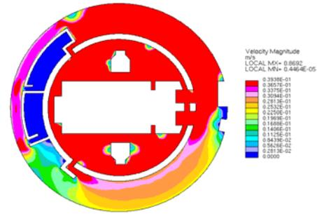
Fig. 2 CFD analysis result for small size debris – 0.12 ft/s, 0.0366 m/s (EL. 100 ft 7 inch)
