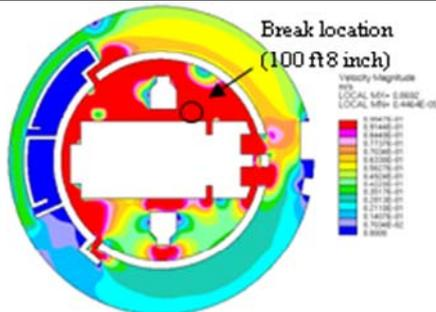
Fig. 1 CFD analysis result for large size debris – 0.30 ft/s, 0.0914 m/s (EL. 100 ft 7 inch)
