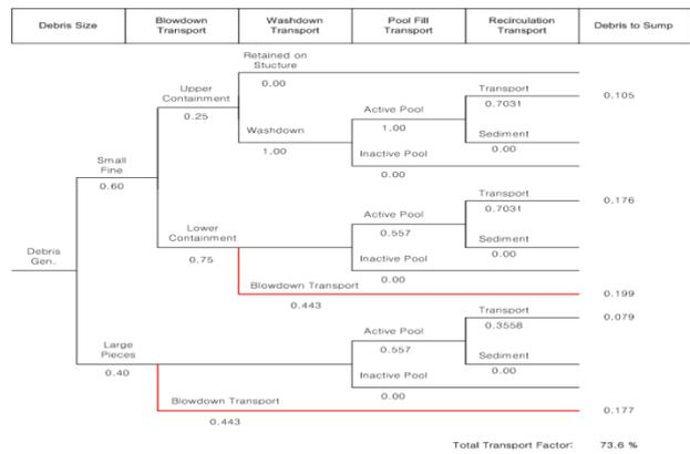
Fig. 3 NUKON transport logic tree for APR1400 plant
