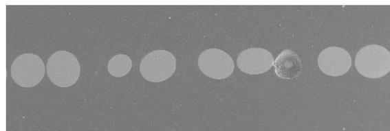
Fig. 4 Morphology of cross section of U-Mo particle arrayed fuel specimen
