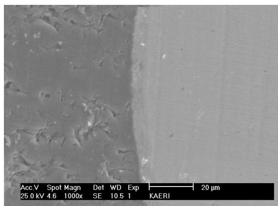
Fig. 3 Interaction between the U-Mo particles and the aluminum matrix
