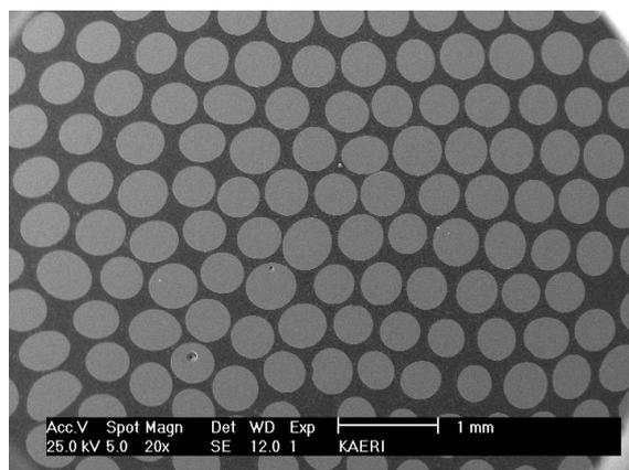
Fig. 2 Transverse section of pressure-sintered sample
