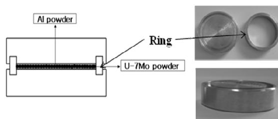
Fig. 1 Compacting Mold
