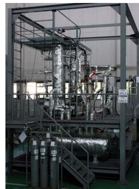
Fig. 2. Sodium-water reaction test facility at KAERI.
