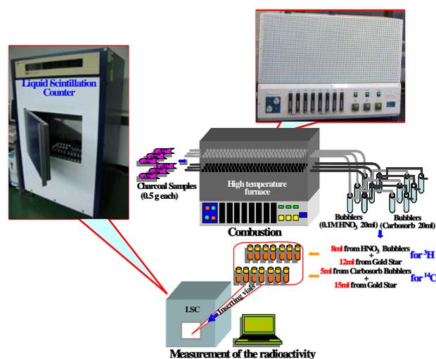
Fig.1. The experimental system for combustion, trap and  $^{14}\text{C}$  radioactivity measurement of the samples.
