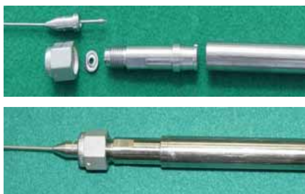
Fig. 3. The End Plug using VCR (before and after assembling)
