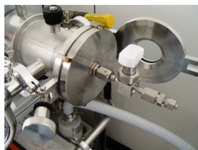
Fig. 4. A Jig for Helium Leak Test of the End Plug using VCR
