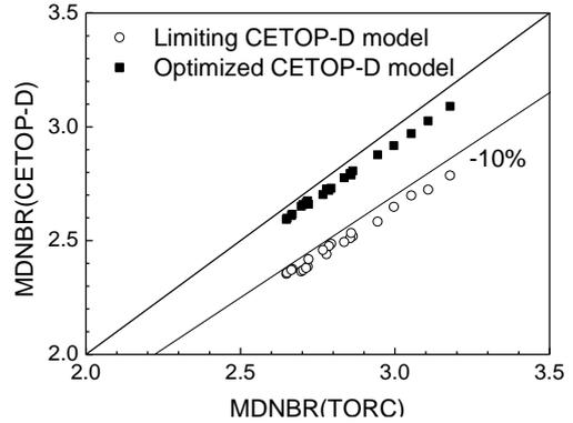
Fig. 3. CETOP-D MDNBR conservatism near a nominal operating condition.
