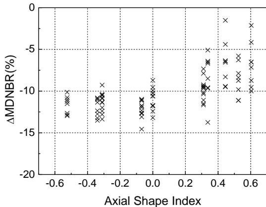
Fig. 2. MDNBR difference depending on axial shape index.
