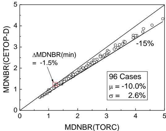
Fig. 1. Comparison of the CETOP-D and TORC MDNBR.
