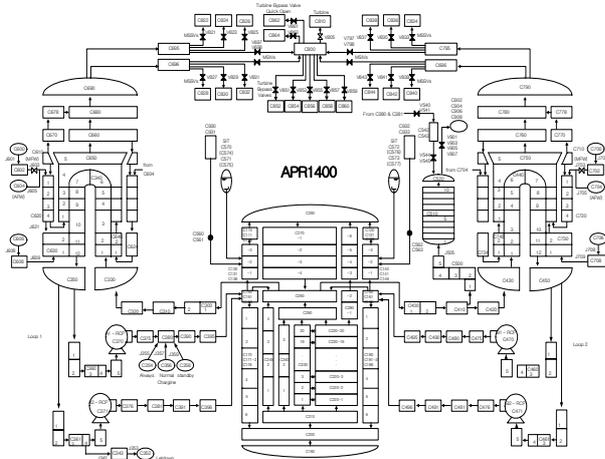
Fig. 2 Nodalization of APR1400
