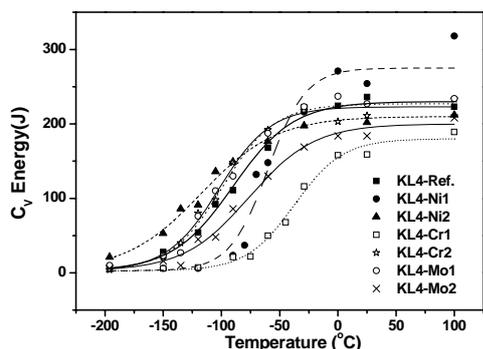
Fig.3. Variation of Charpy impact energy in the temperature range from -196°C to 100°C.
