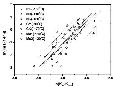
Fig. 2. Master curve for the fracture toughness test results of SA508 Gr.4N model alloys
