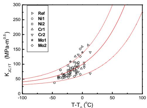
Fig. 1. Master curve for the fracture toughness test results of SA508 Gr.4N model alloys
