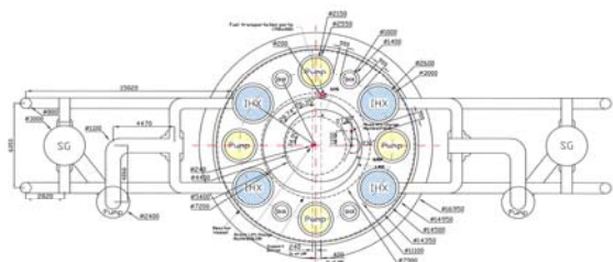
Fig. 2. NSSS arrangement of two-loop system of a pool type SFR of 1200MWe.
