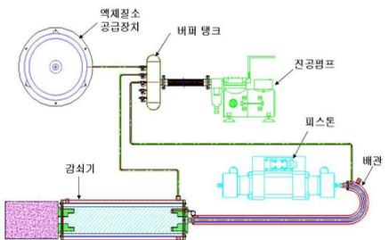
Fig. 4. Figure of LN2 supply equipment and vacuum generation equipment.
