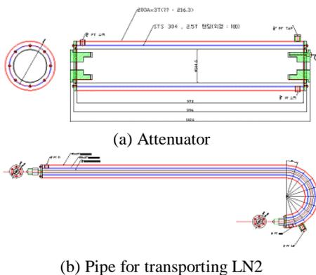
Fig. 5. Figure of cryogenic cooling system of attenuator and pipe for transporting LN2.
