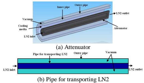
Fig. 1. Cryogenic cooling system of attenuator and pipe for transporting LN2.
