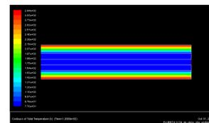
Fig. 3. CFD simulation results of the LN2 transporting pipe.
