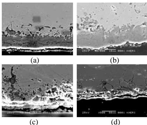
Fig. 4 The morphology of cross section in the gas phase of sulfuric acid for 30days
