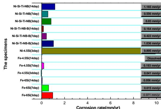
Fig.1 The corrosion rates in the boiling sulfuric acid
