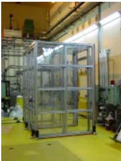
Fig. 2 The outer shape of radioactive substance contamination diffusion preventive equipment for a hot cell located in a intervention area of IMEF.
