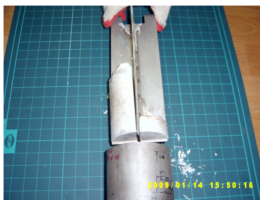
Fig.3.Photograph of a LiCl-KCl molten salt pellet in the mold
