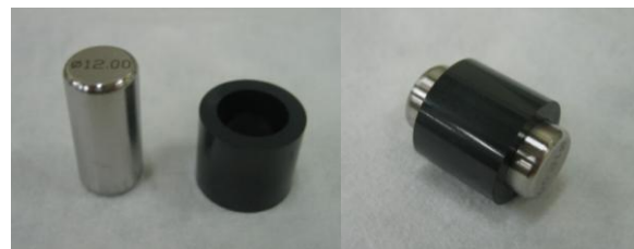
Figure 1. The annular compact which the tungsten metal rod was inserted (before CIP).
