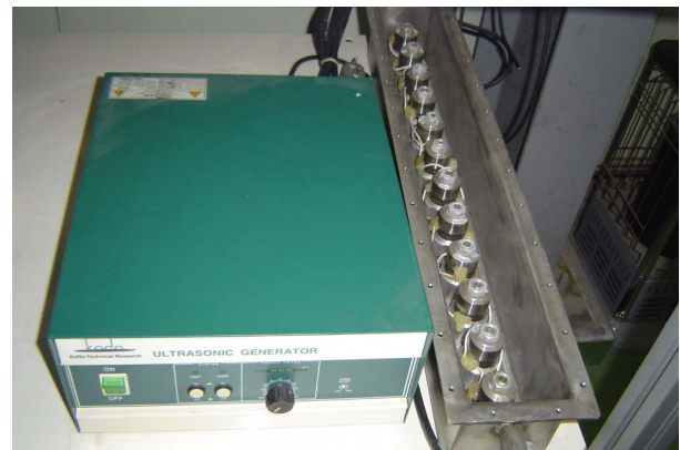
Fig. 1. Piezoelectric Transducers and Power Supply
