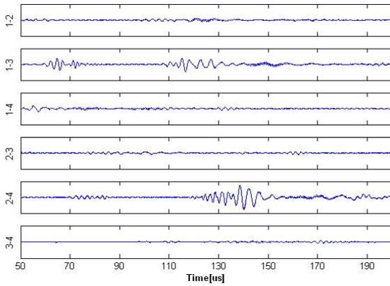
Fig. 3. Differenced signals from all transducer pairs between defected specimen and undamaged specimen
