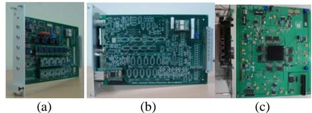
Fig. 2. (a) Pulser/receiver module (b) communication module (c) ADC & main controller module
