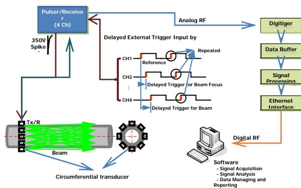
Fig. 1. Schematic diagram of online structural health monitoring system for the structures in a nuclear power plant
