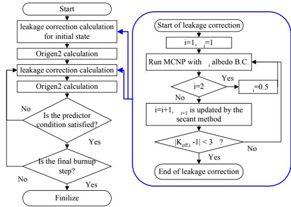
Fig. 1. Flow chart of leakage corrected spectrum depletion in the modified MONTEBURNS code
