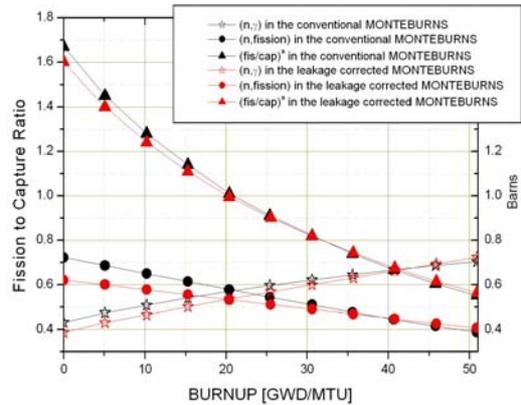
Fig. 5. Fission to capture ratio and one group cross-sections in fuel material vs. burnup
