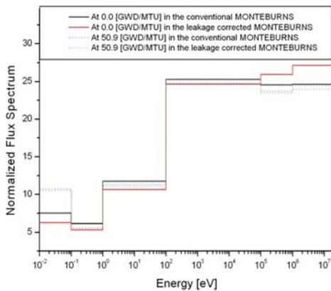
Fig. 4. Normalized neutron flux spectra in two burnup stages
