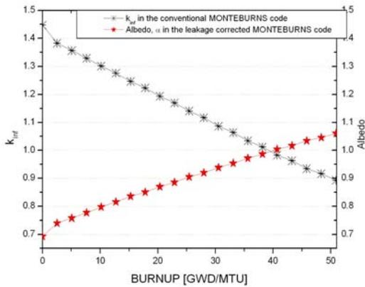
Fig. 3. Trend of  $k_{inf}$  and albedo vs. burnup
