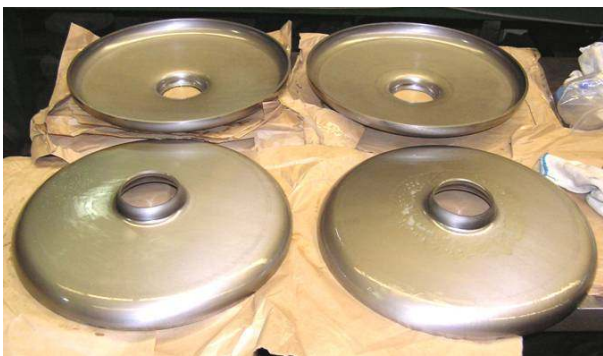
Figure 4. Half-cell after deep drawing.
