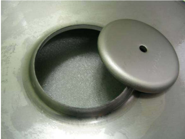
Figure 3. Broken part of half-cell during deep drawing.
