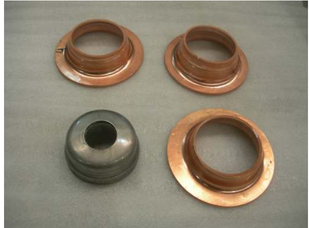
Figure 6. Beam-pipe transition part after deep drawing.
