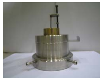
Fig. 1 A jig for dispersing U-Mo large particles
