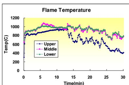
Fig. 4. Flame temperature during the thermal test
