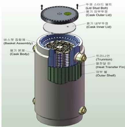
Fig. 1. Configuration of KN-18 Shipping Cask..
