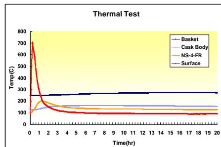
Fig. 5. Temperature profile during the thermal test
