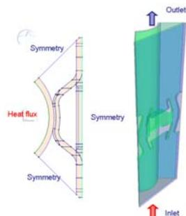
Figure 3. Boundary Conditions of CFD Analysis Model
