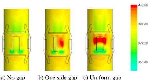
Figure 4. Temperature Distributions on the Fuel Rod Surface with Different Gap Conditions
