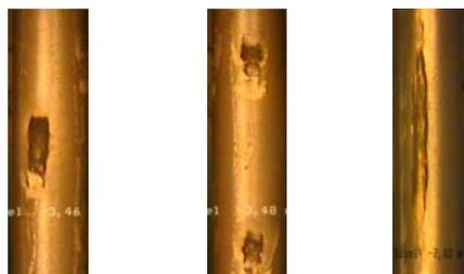
Figure 1. Thick Corrosion Layers found at Contact Surface with Grid Spring and Dimple
