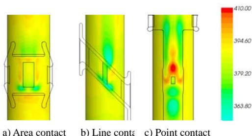
Figure 5. Temperature Distributions on the Fuel Rod Surface with Different Spring Contact Configurations
