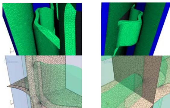
Figure 2. Mesh Configuration of Spring(left) and Dimple(right)
