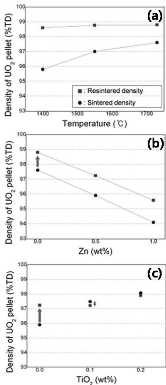
Figure 3. The density change after re-sintering  $UO_2$  pellets; (a) Pure  $UO_2$  (b) Zinc stearate doped  $UO_2$  (c) 0.5wt% Zinc stearate +  $TiO_2$  doped  $UO_2$
