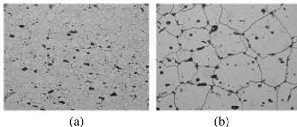
Figure 2. The grain structure of ADU  $\text{UO}_2$  pellets( $\times 200$ )
