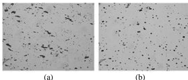
Figure 1. The pore structure of ADU  $\text{UO}_2$  pellets( $\times 200$ )
