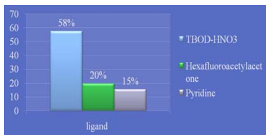
Fig. 5. Extraction efficiency of uranium from mock-up soil by TBOD, HFA, Pyridine in Sc-CO 2
