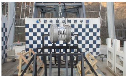
Fig. 1. Spent Resin Transport 1/3 scale model
