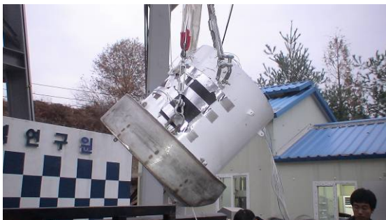
Fig. 7. Deformed shape after C.O.G drop
