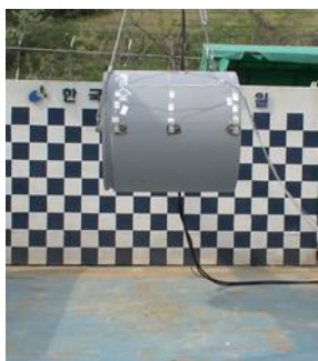
Fig. 6. Horizontal drop test with 1.2 m drop height
