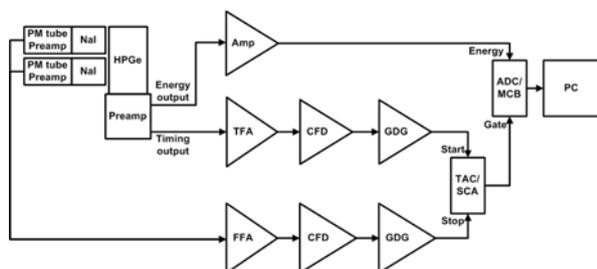
Fig. 1. Block diagram of the Compton suppression system using a HPGe and two NaI(Tl) detectors.
