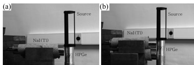
Fig. 2. Arrangement of Compton suppression system using one HPGe and one(a) or two(b) NaI(Tl) detectors.
