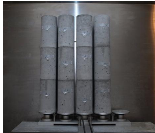
Photo 1. Layout of the \gamma -irradiation test
