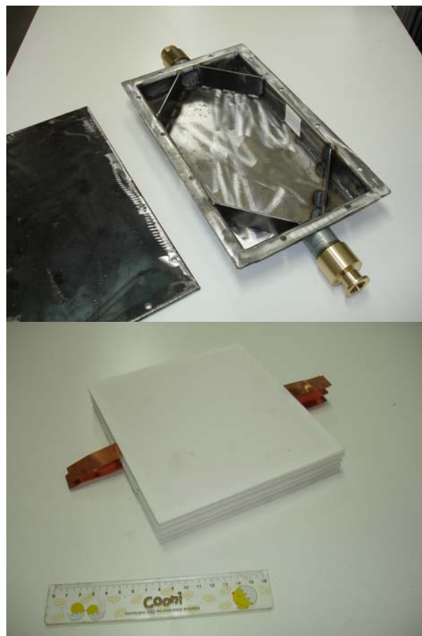
Fig. 4 Pictures of the dielectric barrier discharger components.
