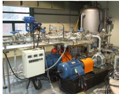
Fig. 1 Experimental Setup for Pump Performance Test
