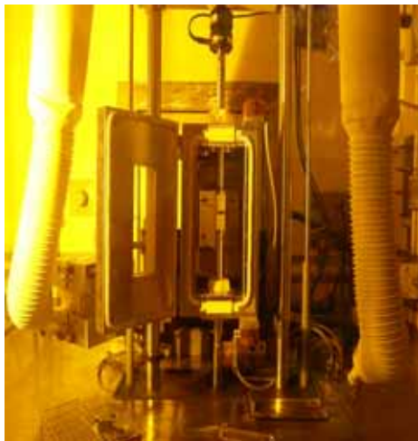
Fig. 2. Experimental apparatus for ring compression test in a hot cell
