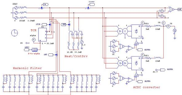
Figure 2. The main circuit for RPC and the loads.
