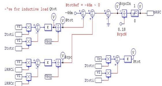
Figure 1. The circuit for  $P_{tot}$ ,  $Q_{tot}$ , and  $BrpcIn/BrpcN$ .
