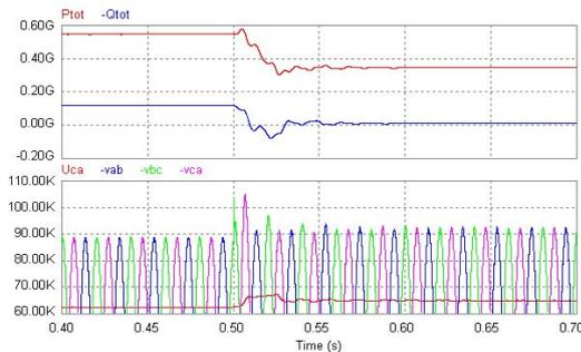
Figure 3. The powers  $P_{tot}$ ,  $Q_{tot}$  (top plot), the rms voltage  $U$ , and the voltage waveforms (bottom plot) when HC is cut off.  $S_g = 10\text{GVA}$ ,  $Q_{totRef} = 0$ .
