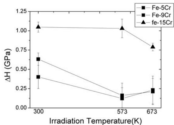
Figure.1. The change of nano hardness in Fe-Cr alloys with irradiation temperature.
