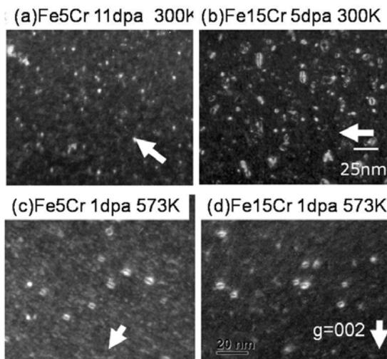
Figure 2 Dislocation loop structures in ion irradiated Fe-5Cr and Fe-15Cr alloys
