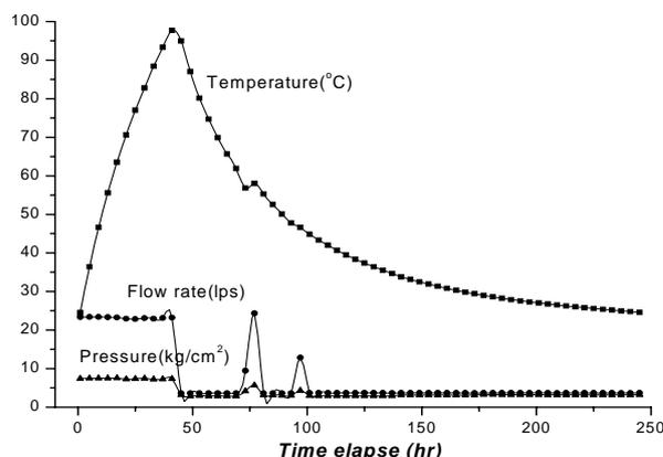
Fig. 2. Graph of 1<sup>st</sup> baking temperature
