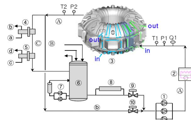
① cooling & baking pipe ② baking pipe ③ cooling pipe ④ circulation pump ⑤ electric heater ⑥ vacuum vessel ⑦ pre-cooler ⑧ cooler ⑨ storage tank ⑩ polishing system ⑪ u.v system ⑫, ⑬ cooling & baking on-off valve ⑭ cooling tower water supply (32°C) ⑮ return (37°C) ⑯ chilled water supply (7°C) ⑰ return (12°C)
