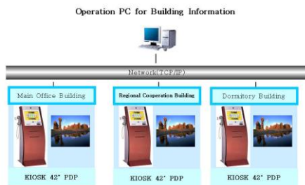
Fig. 3. Configuration of building information system
