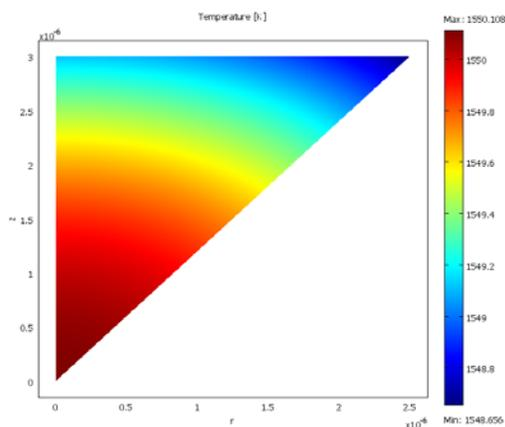
Fig. 2. Axial-symmetric temperature profile of the conical target portion.
