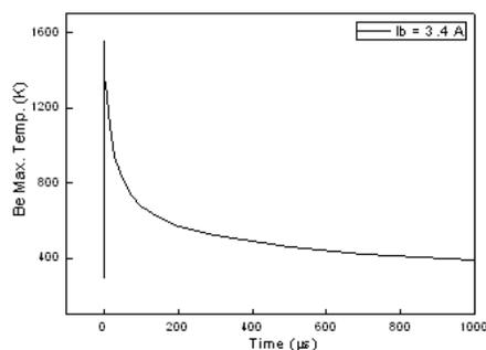
Fig. 3. Max. Be temperature as a function of time in  $\mu\text{s}$ .
