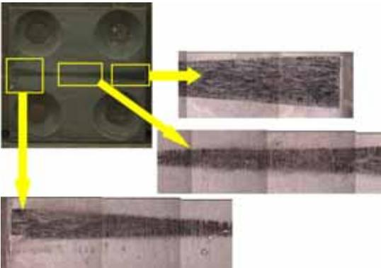
Fig. 4. Worn surfaces of carbon steel support plate
