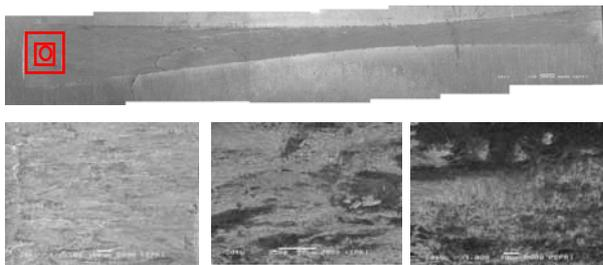
Fig. 5. Worn surface of alloy 600 against carbon steel
