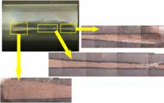
Fig. 3. Worn surfaces of alloy 600 tube
