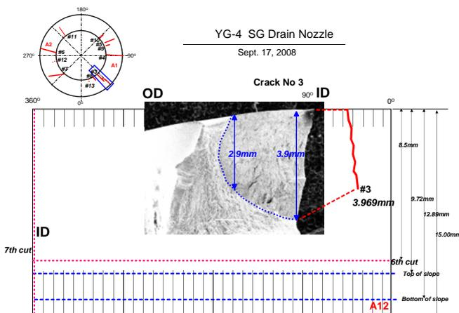
Fig. 5 Location and depth of the no. 3 crack
