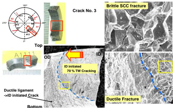
Fig. 4 Feature of cracks developed on the nozzle
