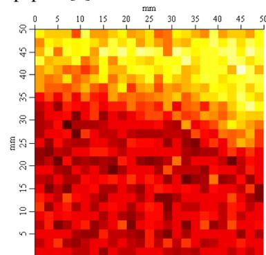
Fig. 3 EMAT C-scan image of the sample
