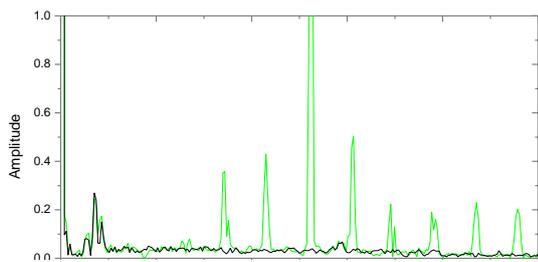
Fig. 4. Signal Spectrum at the good bond and delaminated position
