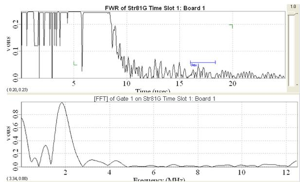
Fig. 2 Typical zoomed waveforms at a delaminated position
