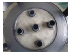
(a) Point A (b) Point B Fig. 5. Picture of the Plenums after Sulfuric Acid Experiment
