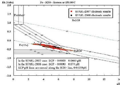
Figure 1. Measured ECP and pH at the carbon steel specimen
