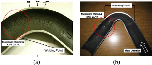
Figure 2. Destructive test result: Inner Surface (a) SFASL-2007 (b) SFASL-2008
