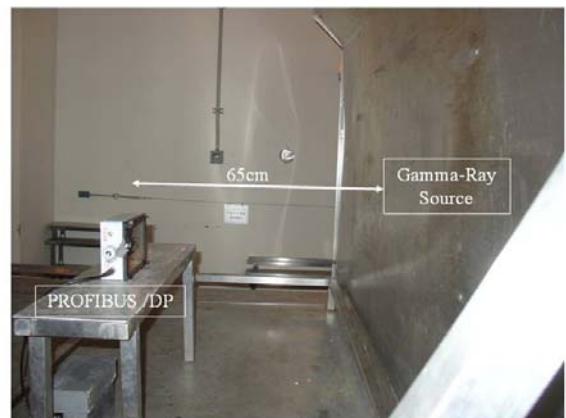
Fig. 3. A profibus/DP field bus communication module placed in the high dose-rate gamma irradiation facility.
