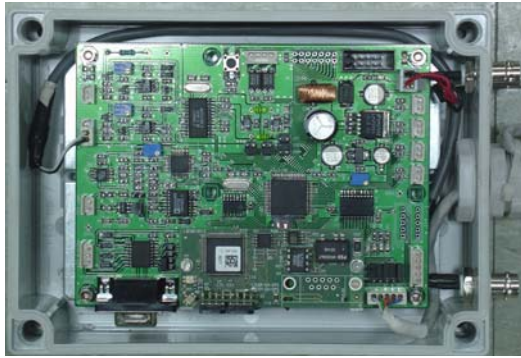
(a) Profibus/DP communication module
