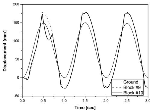
Fig. 5. Displacement history of blocks #9 and #10 in the case without pins and sockets
