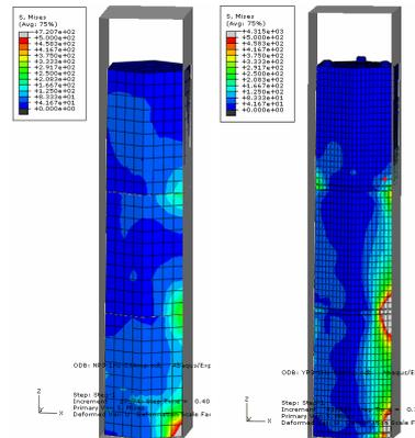
Fig. 2. Overall behavior comparison of the 3-story stacked block structure w/ and w/o pin and socket
