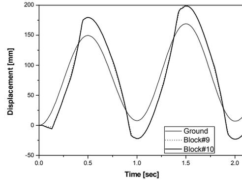
Fig. 6. Displacement history of blocks #9 and #10 in the case with pins and sockets
