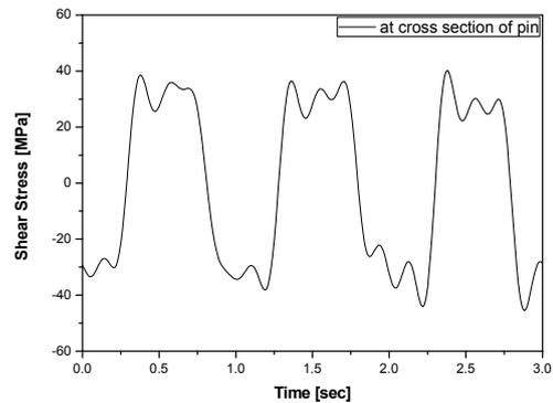
Fig. 3. Shear stress applied to a pin in the lowest block
