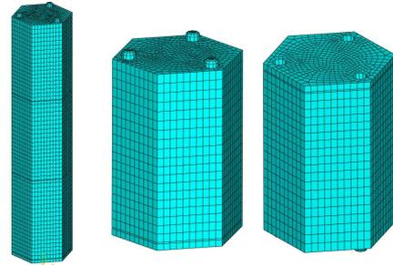
Fig. 1. FE model of the 3-story one-column stacked block
