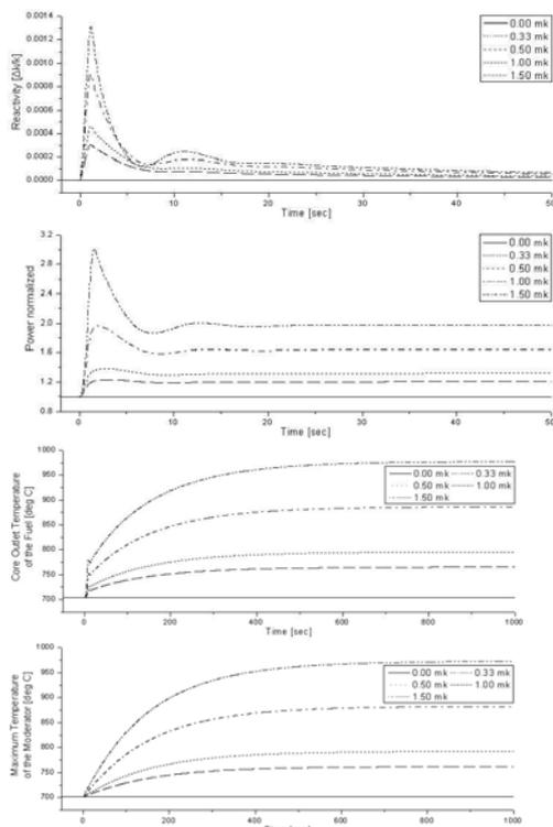
Fig. 3 Reactivity Insertion Transients
