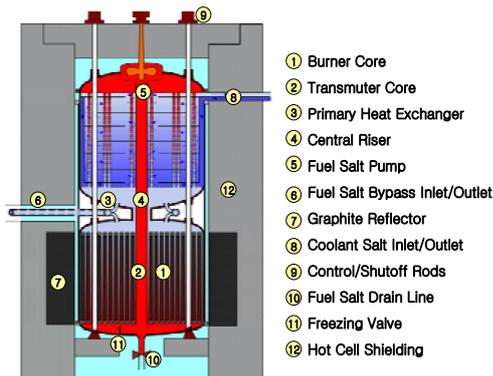
Fig 1. AMBIDEXTER Integral Reactor System
