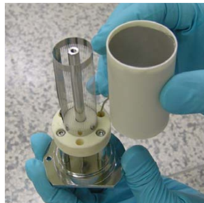
Fig. 3. The inner view of the fabricated HPXe ionization chamber with a shielding mesh.
