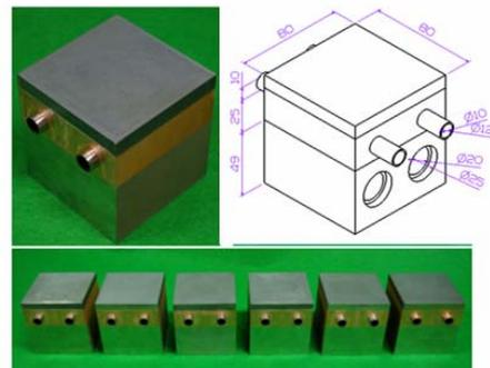
Figure 1 Schematic of the Cu/SS mock-up and its fabrication procedure
