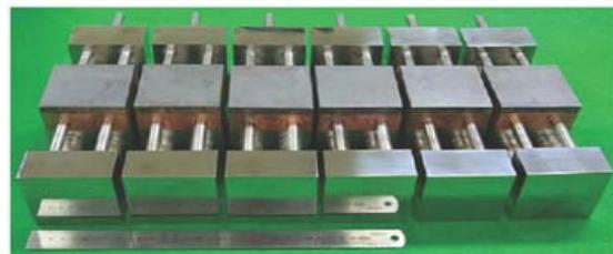
Figure 2 Fabricated mock-ups with manifolds
