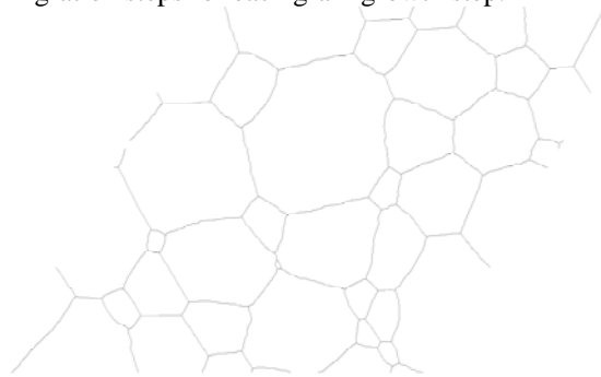
Fig. 1. As-sintered microstructure for a Potts model
