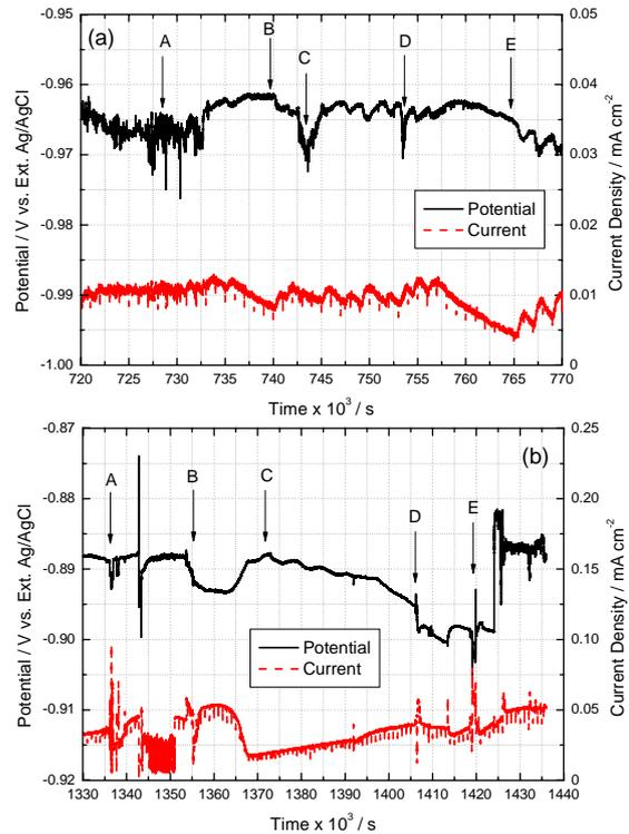
Fig. 1. Time records of the EPN and ECN measured from the stressed C-ring specimens (a) in the solution containing PbO from 720,000 to 770,000 s, and (b) in the solution containing both PbO and CuO from 1,330,000 to 1,436,000 s, respectively.
