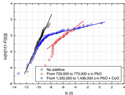
Fig. 2. Plots of  $\ln\{\ln[1/(1-F(t))]\}$  vs.  $\ln t$  determined using the sets of  $f_n$  for the stressed C-ring specimens in the same time region of Fig. 1. The plot obtained for unstressed wire specimen in a 40 wt% NaOH solution without impurities at 290 °C is also given in figure.
