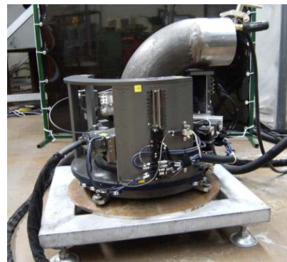
Figure 3. The Weld Overlay System
