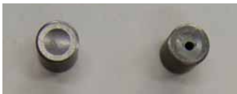
Fig. 2. Fuel pellets (left: before drilling, right: after drilling)
