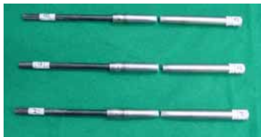
Fig. 4. tensile test of claddings after weld
